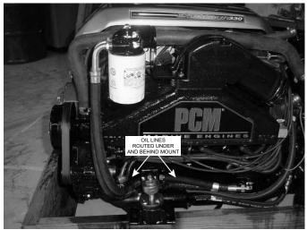
Figure 1-12 Oil Line Routing
