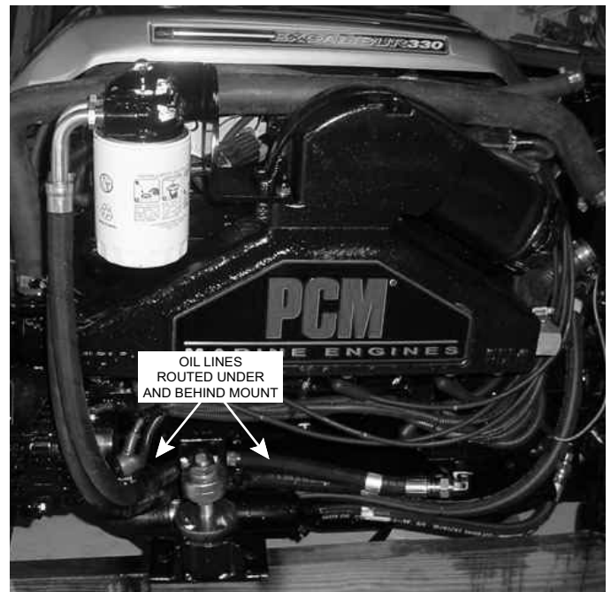
Figure 1-8 Oil Line Routing
